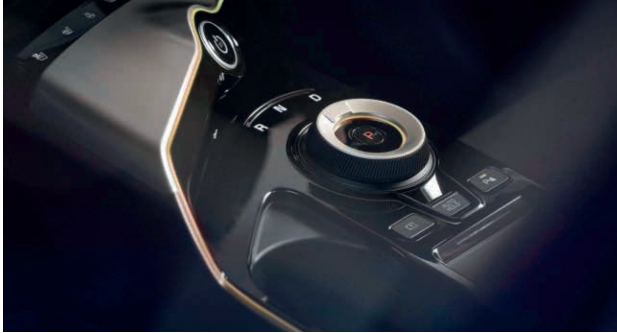
Shift By Wire. All you need to do to change gears between Reverse, Neutral and Drive is brake and turn the dial of the Shift by Wire system left or right. The P button puts the Kia EV6 in Park mode.
